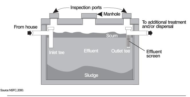
Figure 1-2. Typical single-compartment septic tank with at-grade inspection ports and effluent screen
